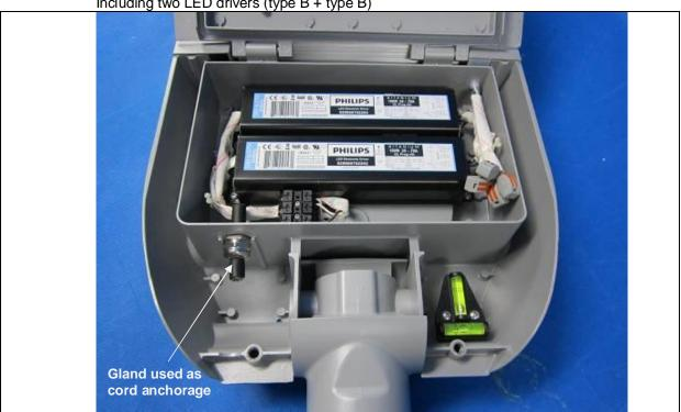
Details of: LED driver view (type A)
