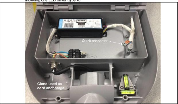
Internal view for models SL-SLA90, SL-SLA120, SL-SLA150, SL-SLB120 and SL-SLB160 Including one LED driver (type B) Details of:
